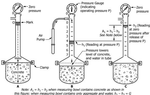
(aggregate correction factor).  $A_1 - G = A$  (entrained air content of concrete)
