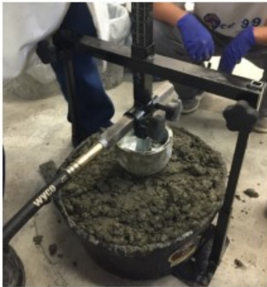
Figure 2 —Depth of Penetration under Static Load (Source: National CP Tech Center)
